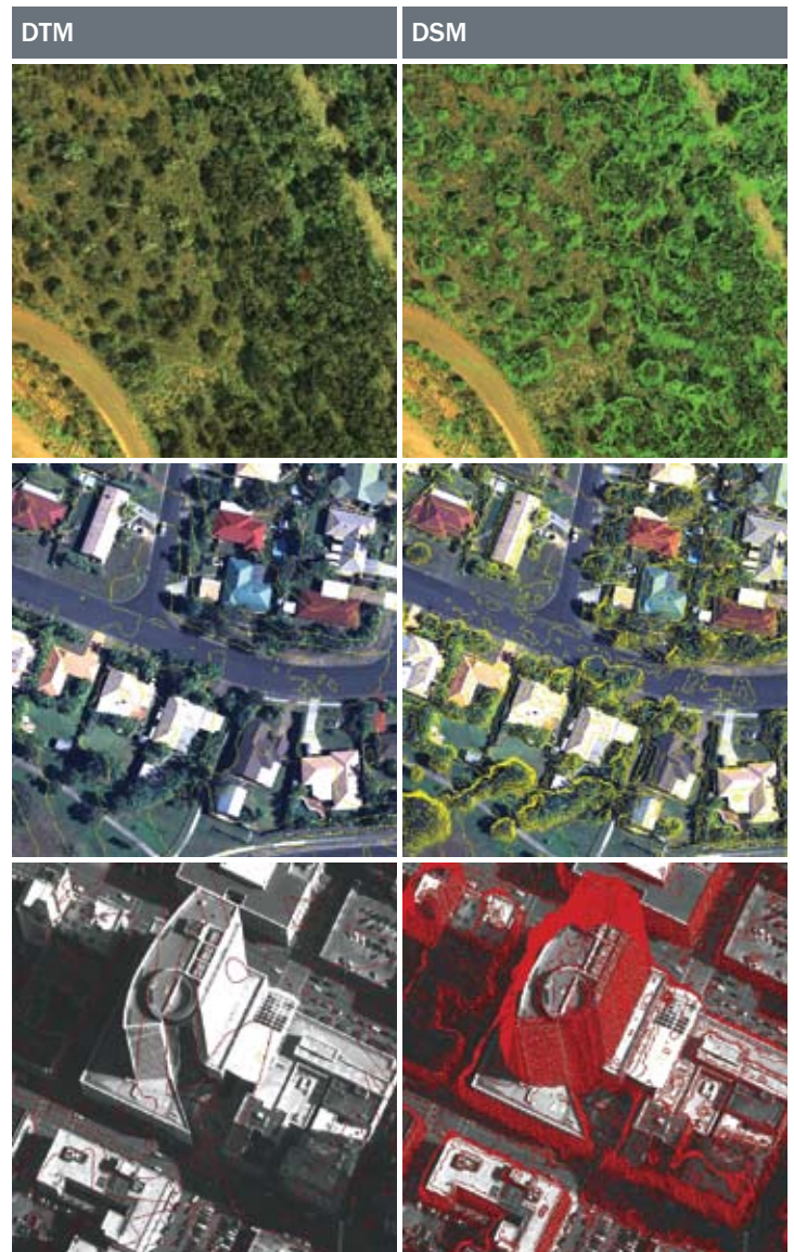
NGATE creates DTMs/DSMs simultaneously. Top and center image pairs courtesy of AAMHatch. Bottom image pair courtesy of HJW GeoSpatial.
