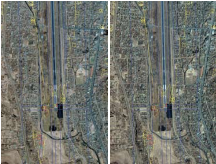
Stereo IKONOS image pair with superimposed graphics identifying areas of interest for interactive extraction and attribution of vertical obstructions. IKONOS images courtesy of GeoEye.
