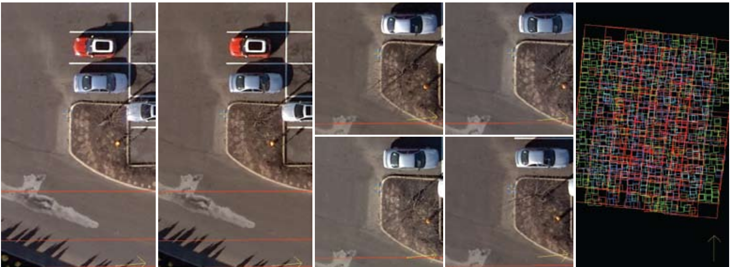
Multiple image display for manual and semi-automatic point measurement and review, including graphics for diagnosis of the overall triangulation solution.
