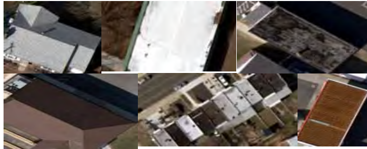
Figure 1. Six different building colors and patterns For example, the supervised building region growing classification would need six signatures. Two (upper-right and lower-middle) of the signatures cannot be used because they are not very homogeneous. These six buildings are from one image (7500 x 11500) with a GSD of 0.14 feet.
