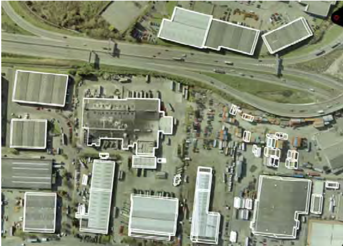
Figure 4. Case study one AFE extracted 59 buildings and 13 trees. White lines are building boundaries. Yellow dots are trees (yellow dots are very small to see). The root mean square error of building boundaries is about 0.2 meters or one post spacing.
