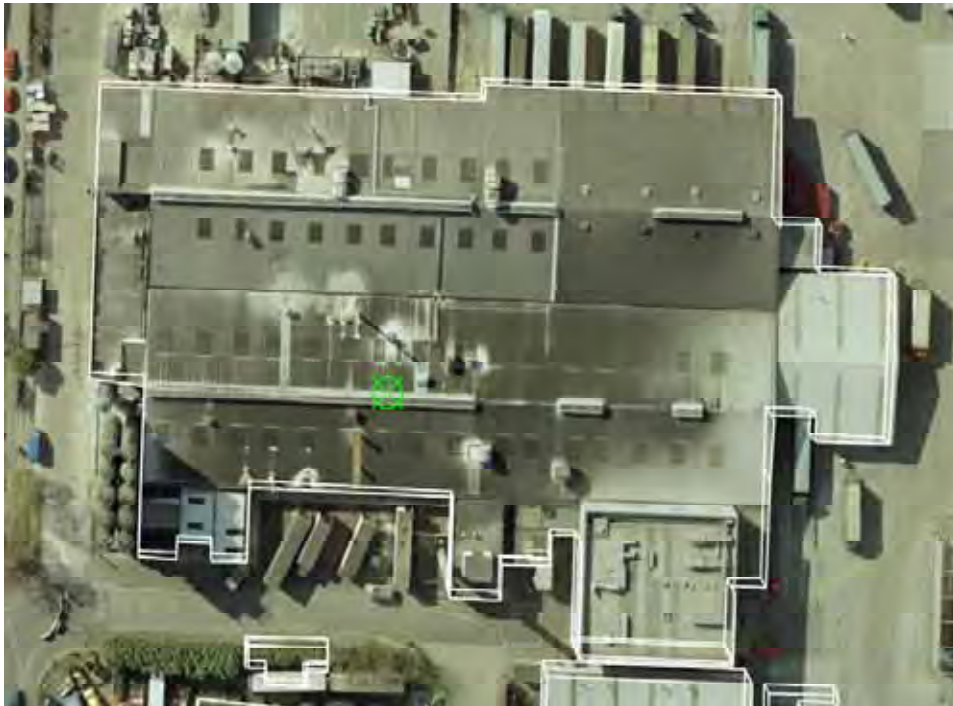
Figure 5. A complex building with more than 50 sides Only LIDAR point cloud was used to extract this complex building. Stereo images are used only to verify the accuracy of the extracted building. With very dense and accurate LIDAR point clouds like this, AFE can extract 3-D side models accurately.
