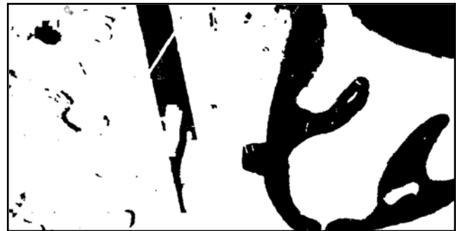
Figure 6: Result of graph-cut optimization to produce spatially coherent regions. Notice how the pixels that would have been spuriously labeled near the sandbar and on the land areas are cleaned. The details of the bridge, docks and water vehicles are preserved.
