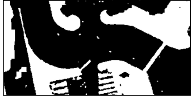
Figure 5: Spatially coherent regions extracted after applying graph-cut optimization. Black regions denote water areas. The docks and water vehicles are preserved, while spuriously classified pixels are accurately incorporated into either the land or water regions.
