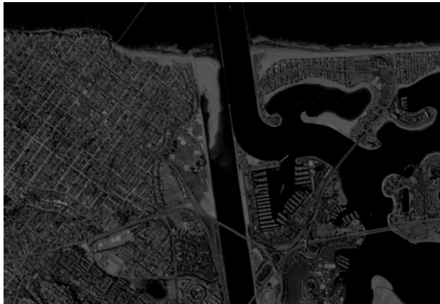
Figure 3: For the harbor data, this image depicts the difference at each point between the spectral signature of the pixel and the spectral signature of the seed. Low intensity values signify proximity in spectral feature space to the seed pixel.
