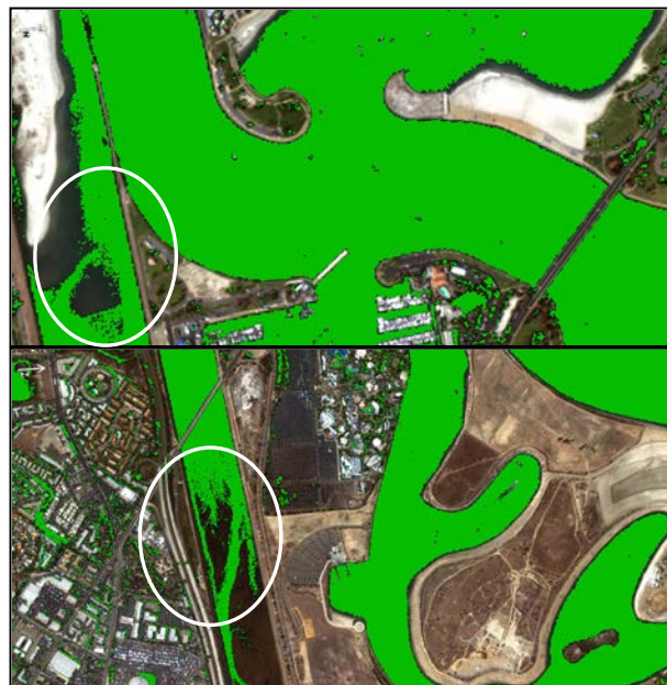
Figure 2: The above two areas show the result of simply classifying the water areas by spectral classification and then using a threshold to denote interior (green areas) vs exterior. The circles highlight areas containing many spurious classifications.
