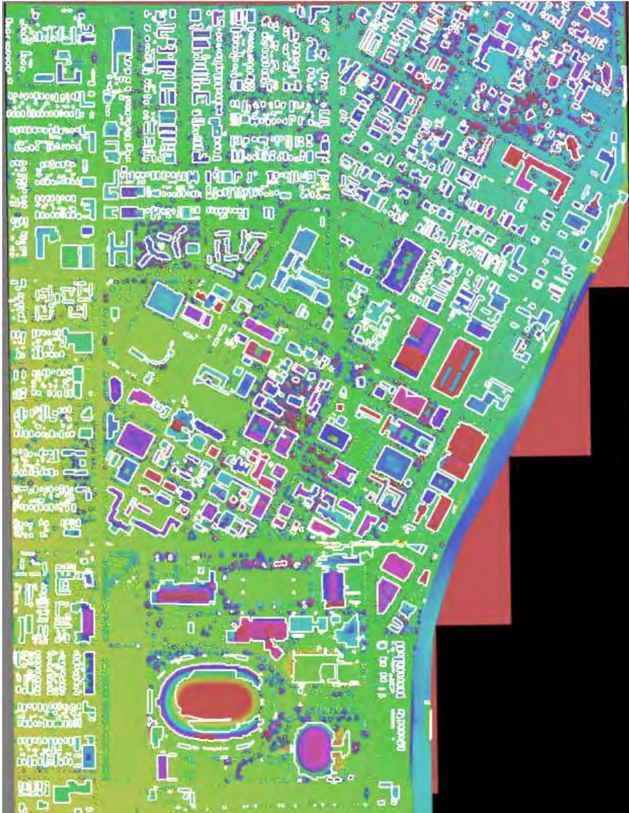
Figure 13. AFE extracted 2464 buildings/houses (white lines) and 5164 trees (yellow dots).
