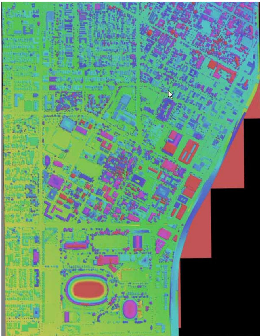
Figure 12. Terrain shaded relief covers 24.8 square kilometers of the USC campus. The area is relatively flat and the transformation from DSM to DEM is easier than the Allegheny County area. AFE cannot extract buildings such as the football stadium and the track field. There are many trees. It is a challenge when trees overhang a building or are attached to a building with similar height. There is no LIDAR data in the lower right corner area, which is either black or uniformly red.
