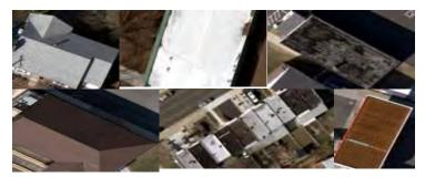
Figure 1. Six different building colors and patterns For example, the supervised building region growing classification would need six signatures. Two (upper-right and lower-middle) of the signatures cannot be used because they are not very homogeneous. These six buildings are from one image (7500 x 11500) with a GSD of 0.14 feet.
