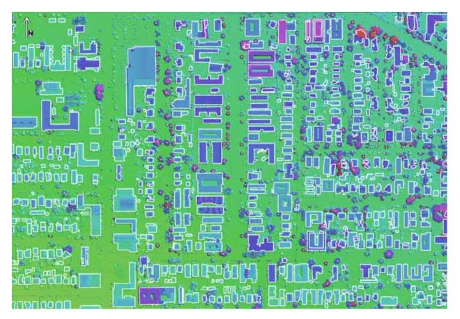
Figure 16. Buildings and houses with parallel or perpendicular sides Buildings and houses with parallel or perpendicular sides are easy 3-D features for AFE. However, AFE may still have difficulty when the buildings and houses are less than 3 meters in height. Low 3-D features are difficult for the DSM to DEM transformation.
