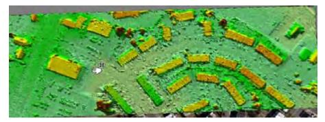
Figure 2. Terrain shaded relief of a point cloud 3-D objects are immediately apparent. Their locations and their approximate shapes are obvious. It is much easier to classify a TSR for 3-D objects than to classify digital images. The six buildings in Figure 1 are shown in this figure.
