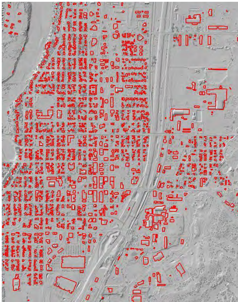
Figure 22. Redmond, Oregon. This LiDAR dataset has 39 million points covering an area of 4.9 km 2 . The background image is terrain shaded relief generated from a 0.59 foot gridded DSM. 1780 houses and buildings were extracted by AFE with a success rate of 92%. Most of the incorrectly extracted houses and missing houses are due to overhanging trees.
