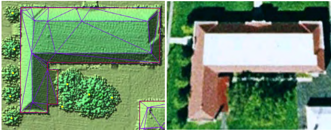
Figure 10. AFE uses a 3-D mesh to model a complex roof. On the right is an image captured from Google Earth at 44° 18' 08.64" N, 120° 50' 25.53" W. Purple lines are 3-D meshes. Red lines are the rooftop polygon. Yellow dots are trees. Image © 2012 DigitalGlobe and 2012 Google.
