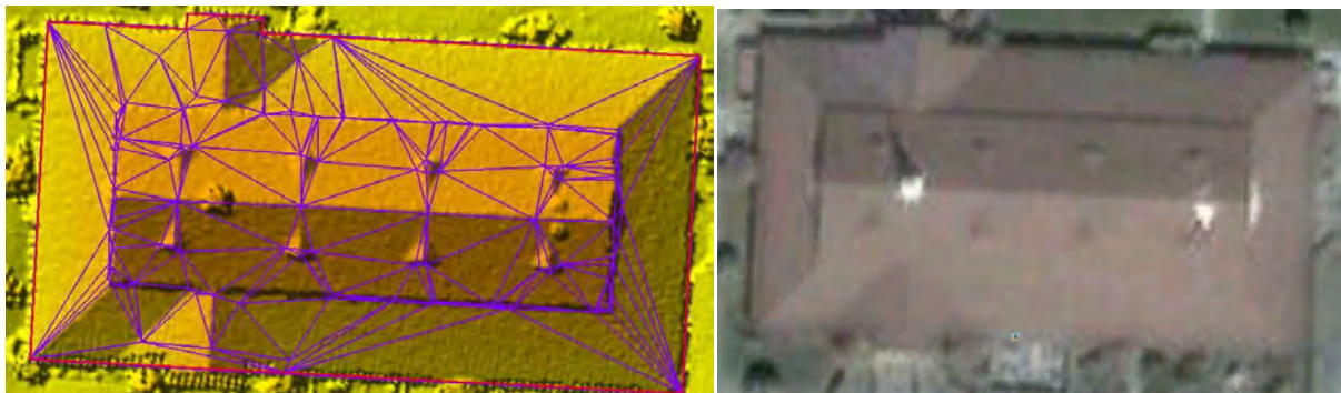
Figure 18. North Bend, Oregon. AFE uses a 3-D mesh to model a complex roof. On the right is an image captured from Google Earth at 43° 24' 24.16" N, 124° 15' 15.67" W. Purple lines are 3-D meshes. Red lines are the rooftop polygon.
