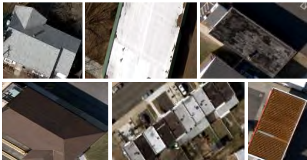
Figure 1. Six different building colors and patterns. A supervised building region growing classification would need six signatures. The upper-right and lower-middle signatures cannot be used because they are not homogeneous.
