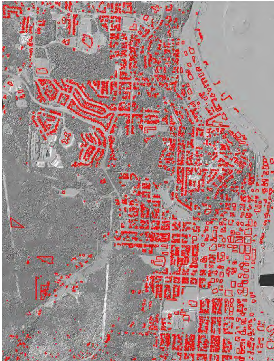
Figure 19. Coos Bay, Oregon. This LiDAR dataset has 73 million points covering an area of 9.1 km 2 . The background image is terrain shaded relief generated from a 0.59 feet gridded DSM. 3812 buildings were extracted by AFE with a success rate of 87%. Most of the incorrectly extracted and missing buildings are due to overhanging trees.
