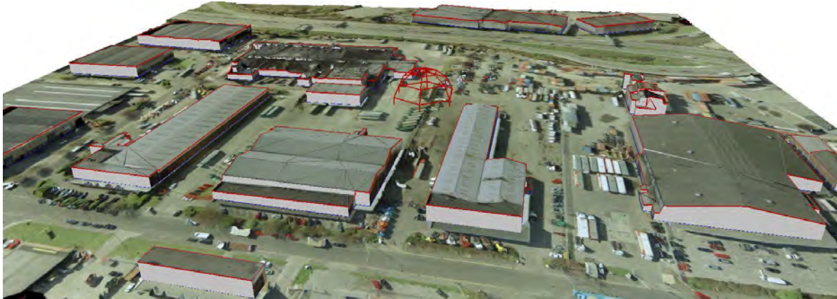
Figure 25. Fully textured 3-D view of Bristol, U.K. The buildings were extracted by AFE using dense and accurate LiDAR point clouds. Stereo images and LiDAR point clouds were accurately registered. SOCET GXP Auto Texture was used to apply textures to the buildings. The whole process is automated without any manual editing.
