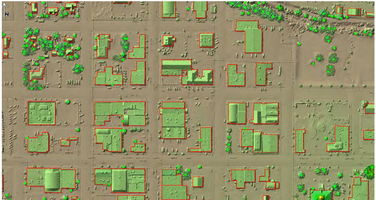
Figure 8. There are a total of 52 buildings. AFE extracted 49 buildings and houses correctly. Two houses were extracted incorrectly and one house is missing. AFE achieved a success rate of 92%. The two incorrect houses are due to overhanging trees. The missing house is due to the size of the house being too small. These three errors are all in the upper-left corner where there are tall trees.
