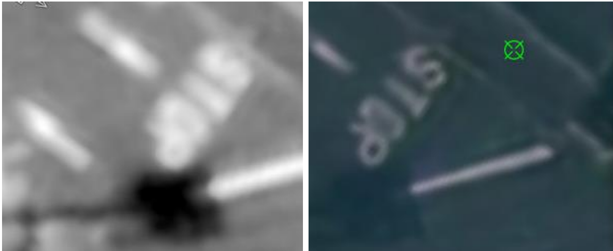
Figure 5. Super-resolution images make searching and recognizing man-made objects easier. The right image is 15cm GSD, satellite MSI, deduced from the 30cm GSD pan-sharpen image on the left. The letters are much easier to recognize in the super-resolution image. CNN based super-resolution networks use AI to learn the transformations from lower resolution images to higher resolution images. Image © 2021 Maxar Technologies.
