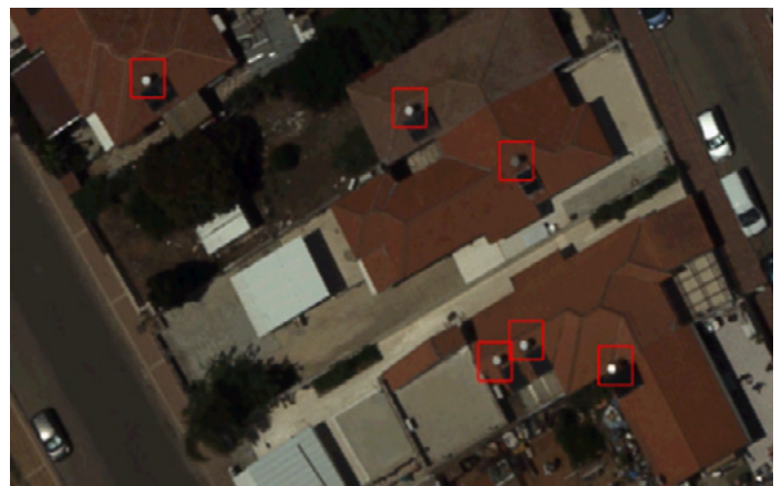
Identification of solar water heaters on rooftops of urban housing.
