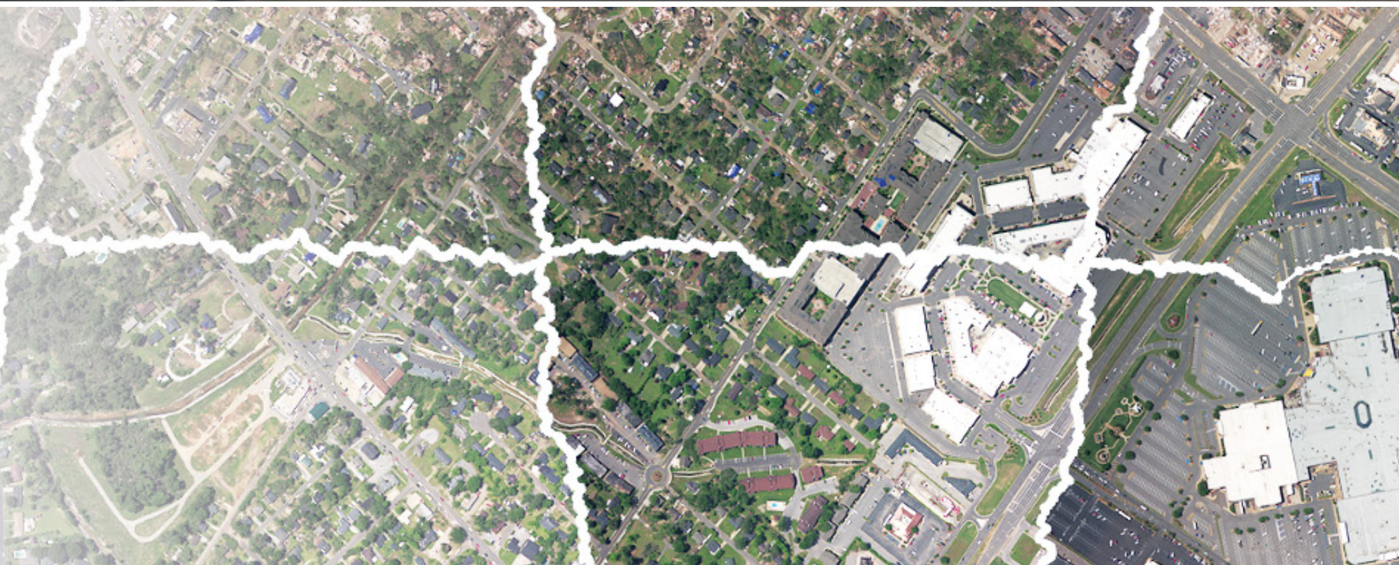
Automatic Feature Extraction (AFE) of buildings from a 0.5m, Next Generation Automatic Terrain Extraction (NGATE) DSM. Imagery courtesy of Ordnance Survey Great Britain.
