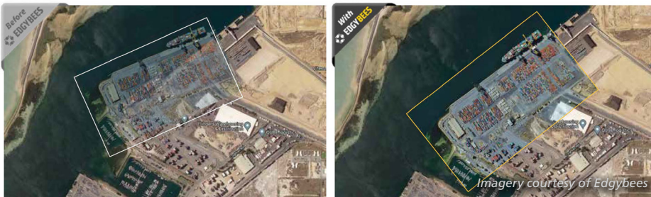
Maxar WorldView-3 satellite imagery correction from an 11m offset (left) to a 2m offset (right) using Edgybees Sky technology for improved accuracy.
